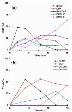
Figure 3. Time course of the Pd/C catalyzed reaction of HMF under H<sub>2</sub> (30 psi). (a): w/o acid. (b): CH<sub>3</sub>CO<sub>2</sub>H (10 equiv). Reaction conditions: substrate (0.5 mmol), substrate/Pd = 10 molar ratio, dioxane (5 mL), 120 °C.
