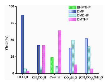
Figure 4. Effect of additives on the conversion of HMF under H<sub>2</sub> (30 psi) with Pd/C catalyst. *Control:* no additive. *Reaction conditions:* substrate (0.5 mmol), substrate/Pd = 10 molar ratio, dioxane (5 mL), 120 °C.
