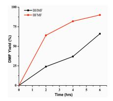
Figure 2. Time course of conversion of BHMF and BFMF to DMF. *Reaction conditions:* substrate (0.5 mmol), substrate/Pd =10 molar ratio, FA (10 equiv), dioxane (5 mL), 120 °C.
