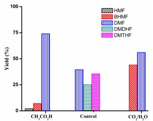
Figure 5. Product distribution for the reaction of HMF with Pd/C (substrate/Pd = 20 molar ratio). *Control:* no additive *Reaction conditions:* substrate (2 mmol), dioxane (5 mL), 120 °C, 15 h.
