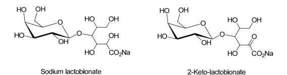
Figure 3. Lactobionate derivatives obtained after the oxidation of lactose.
