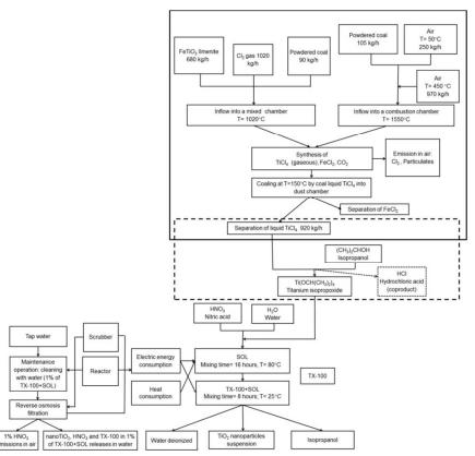
Fig. 1 Bottom-up hydrolytic synthesis of TiO<sub>2</sub> nanoparticles life cycle
