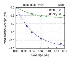
**Fig. 5** Dependence of  $\Delta \Phi$  of Cu(111) on the coverage of weakly chemisorbed (BTAH<sub> $\perp$ </sub>, blue squares) and physisorbed (BTAH<sub> $\parallel$ </sub>, green circles) benzotriazole. The curves are drawn by fitting the data points with polarizable point-dipole model of ref. 32.
