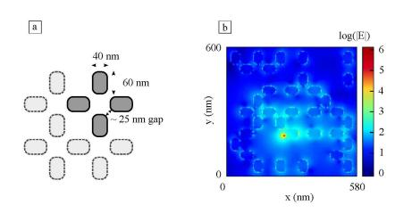
Fig. 3 Panel a) Sketch of the sample structure shown in Fig. 2: each nanoantenna has a size of  $40 \times 60$  nm and the gap between the nanoantenna tips is  $\sim 25$  nm. Panel b) Plot of the electric field intensity at  $\lambda = 720$  nm obtained by FDTD simulations upon dipolar excitation at the location of highest intensity, 7 nm from the closest gold structure. Plasmonic waves of coupled nanoantennas are excited.
