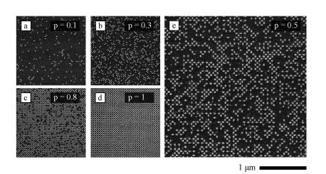
**Fig. 2** SEM images of lithographic gold networks fabricated by EBL on glass substrates. As indicated on the image, panel a) shows the structure for a value of the percolation parameter p = 0.1, panel b) p = 0.3, panel c) p = 0.8, panel d) p = 1, and panel e) p = 0.5. Each element of the network is a nanoantenna of size  $60 \times 40 \times 40$  (L×W×H) nm. Each network is  $10 \times 10 \ \mu\text{m}^2$  and contains  $\sim 10^4$  rods.
