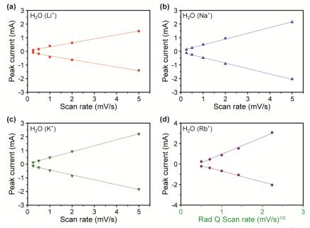
**Figure 6.** The relationship between the peak currents and corresponding scan rates of (a)  $Li^+$ , (b)  $Na^+$ , (c)  $K^+$ , and (d)  $Rb^+$  ions in aqueous electrolytes.
