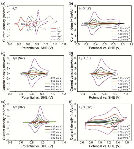
**Figure 5.** CV curves of NiHCFe using the three-electrode Swagelok cell configuration in aqueous electrolytes. The scan rate is 1 mV s<sup>-1</sup>. (a) CV curves of Li<sup>+</sup>, Na<sup>+</sup>, K<sup>+</sup>, Rb<sup>+</sup>, and Cs<sup>+</sup> ions. CV curves of (b) Li<sup>+</sup>, (c) Na<sup>+</sup>, (d) K<sup>+</sup>, (e) Rb<sup>+</sup>, and (f) Cs<sup>+</sup> ions at different scan rates from 0.25 to 5.00 mV s<sup>-1</sup>.
