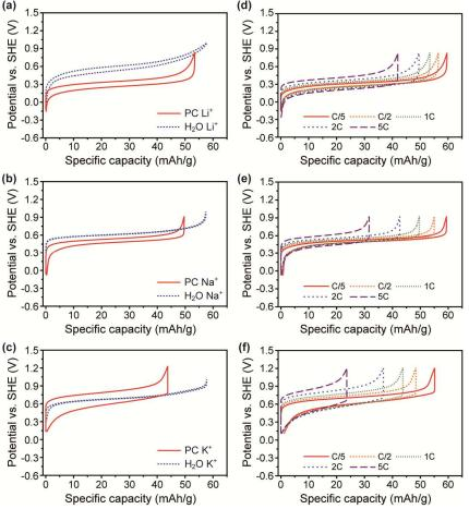
**Figure 3.** Comparison of hysteresis in galvanostatic potential profiles at 1C between aqueous and PC electrolytes. (a)  $\text{Li}^+$ , (b)  $\text{Na}^+$ , and (c)  $\text{K}^+$  ion systems. Typical charge and discharge potential profiles of NiHCFe electrodes at different C rates (0.2, 0.5, 1, 2, and 5 C) with (d)  $\text{Li}^+$ , (e)  $\text{Na}^+$ , and (f)  $\text{K}^+$  ions in PC.
