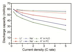
**Figure 4.** Discharge capacity retention in aqueous and PC electrolytes with different insertion ions at varying C rates.
