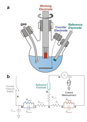
**Fig. 8** Schematic of a three-electrode electrochemical cell. (a) Experimental setup for the three-electrode cell. (b) Circuit of a typical three-electrode cell. In these cells, the potential is measured or controlled between the working and reference electrodes (H), while the current is measured or controlled between the working and counter electrodes (I). The working electrode can be rotated to avoid limitation by transport of the analyte.
