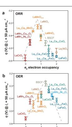
**Fig. 12** The ORR and OER on various perovskite oxides in alkaline solution. (a) Overpotentials for the ORR as a function of  $e_g$  electron occupancy on various perovskites. (b) Overpotentials for the OER as a function of  $e_g$  electron occupancy on various perovskites. Figure adapted from refs. 164 and 67 with permission from Nature Publishing Group and AAAS.
