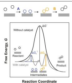
Fig. 3 Schematic illustrations of a prototypical reaction mechanism, transition state theory, and its associated linear free energy relationships. Potential energy
