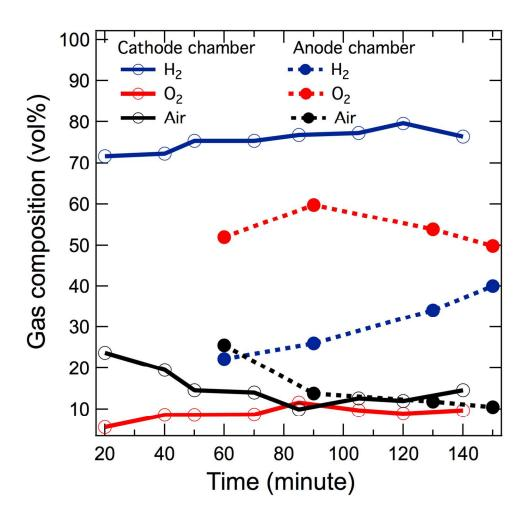
**Figure 4.** Time evolution of the gas composition  $(H_2, O_2 \text{ and air})$  from the cathode compartment (solid lines) and the anode compartment (dashed lines).
