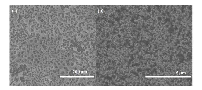
**Figure S4: Top-View Scanning Electron Microscope Images**. Top view SEM image of (a) A capping layer of disperse CH<sub>3</sub>NH<sub>3</sub>SnI<sub>3</sub> crystal formed on an 80 nm thick film of TiO<sub>2</sub>. (b) CH<sub>3</sub>NH<sub>3</sub>SnI<sub>3</sub> coated on a 400 nm thick film of TiO<sub>2</sub> such that all of the crystallites have formed within the pores of the TiO<sub>2</sub> and no capping layer is present.
