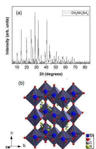
Figure 1: X-ray Diffraction (XRD) and Crystal Structure. (a) XRD pattern derived from a ground powder of CH<sub>3</sub>NH<sub>3</sub>SnI<sub>3</sub>. (b) Simulated crystal structure of CH<sub>3</sub>NH<sub>3</sub>SnI<sub>3</sub> obtained from the diffraction pattern given in (a) showing the tetragonal conformation of the perovskite
