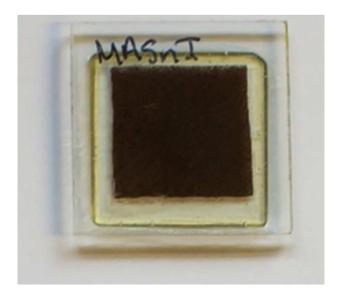
**Figure S1-** Photograph showing a film of the black/brown, CH<sub>3</sub>NH<sub>3</sub>SnI<sub>3</sub>. This film was sealed in a nitrogen filled glove box and has been aged for 4 months under AM1.5 76mWcm<sup>-2</sup> sun light generated from a sun-test CPSPlus light soaking box.
