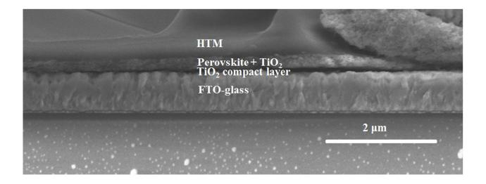
**Figure S3: Cross-Sectional Scanning Electron Microscope (SEM) Image.** Cross-sectional SEM image of a TiO<sub>2</sub>-based CH<sub>3</sub>NH<sub>3</sub>SnI<sub>3</sub> device.
