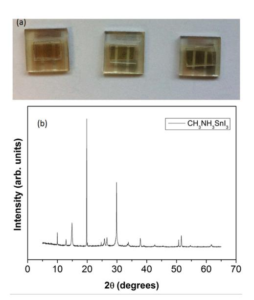
**Figure S2: (a)** Photograph showing solar cell devices where the CH<sub>3</sub>NH<sub>3</sub>SnI<sub>3</sub> absorber layer has degraded. **(b)** X-ray Diffractogram of a degraded sample of CH<sub>3</sub>NH<sub>3</sub>SnI<sub>3</sub>.
