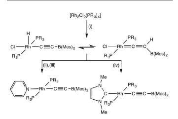
Scheme 1 Braunschweig's synthesis of β-boryl vinylidene and alkynyl complexes  $(Mes = C_6H_2Me_3-2,4,6)$ .<sup>4</sup> (i) H=CBMes; (ii) py; (iii) LiN<sup>i</sup>Pr<sub>2</sub>; (iv) C(NMeCH)<sub>2</sub>.
