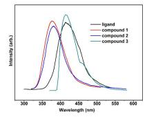
Fig. 5 The solid state emission spectra of  $H_4L$  ligands and MOFs 1–3.
