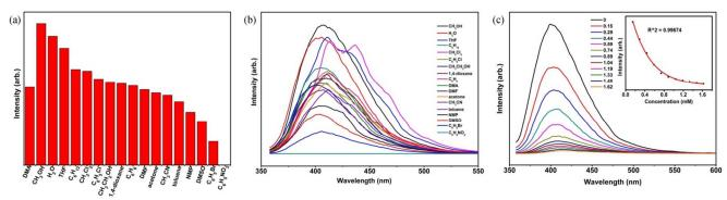
Fig. 7 (a) The relative luminescent intensities of 3 in different solvents; (b) The emission spectra of 3 in different solvents; (c) The luminescent spectra of 3 in DMA with different amounts of NB (Insert: the relationship of the luminescent intensities and NB concentration).
