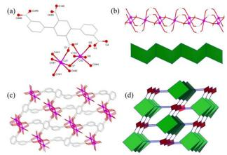
**Fig. 2** (a) The coordination environment of Cd(II) ions in **2**, symmetry codes: #1: 1-x, -y, -z; #2: 1-x, y-0.5, 0.5-z; #3: x, 0.5-y, z-0.5; #4: 1-x, 0.5+y, 0.5-z; #5: 1-x, 1-y, -z; #6: -x, -y, -z. (b) The 1D rod-like SBU formed by Cd(II) ions, hydroxyls and carboxylate groups of L ligands (top) and its simplified net (below). (c) The 3D dense framework of **2**. (d) The topological net of **2**.
