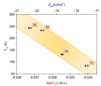
**Fig.5** The plot of spin transition temperature  $T_{1/2}$  of SCO compounds (1ce) as a function of strength of N–H···O contacts quantified either by sign( $\lambda_2$ ) $\rho$  through NCI analysis (red squares) or by the potential energy density  $V(\mathbf{r})$  calculated at BCP points ( $E_{\text{HB}} = V(\mathbf{r})/2$ ) (blue circles).
