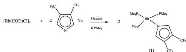
successfully used to synthesize the new complex  $[\text{Rh}(\text{PMe}_3)_3(3,4\text{-(CF}_3)_2\text{-Pyr)}]$  (**1**) (Equation 1). Thus, reaction of a mixture of  $[\text{Rh}(\text{COD})\text{Cl}]_2$  and  $\text{PMe}_3$  with two equivalents of  $3,4\text{-(CF}_3)_2\text{-PyrNa}$  in hexane afforded **1** in high yield (72%). There appear to be few examples of Rh-Pyr complexes where the pyrrolyl moiety is not part of a macrocyclic entity or functionalized with a chelating group.
