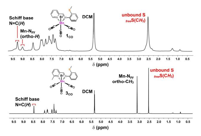
Fig. 5. <sup>1</sup>H NMR spectra (500 MHz) of  $[(\underline{NNS})Mn(CO)_3Br]$  ( $\mathbf{1_{CO}}$ , top panel) and  $[(\underline{MeNNS})Mn(CO)_3Br]$  ( $\mathbf{3_{CO}}$ , bottom panel) in CD<sub>2</sub>Cl<sub>2</sub>. at 25 °C.
