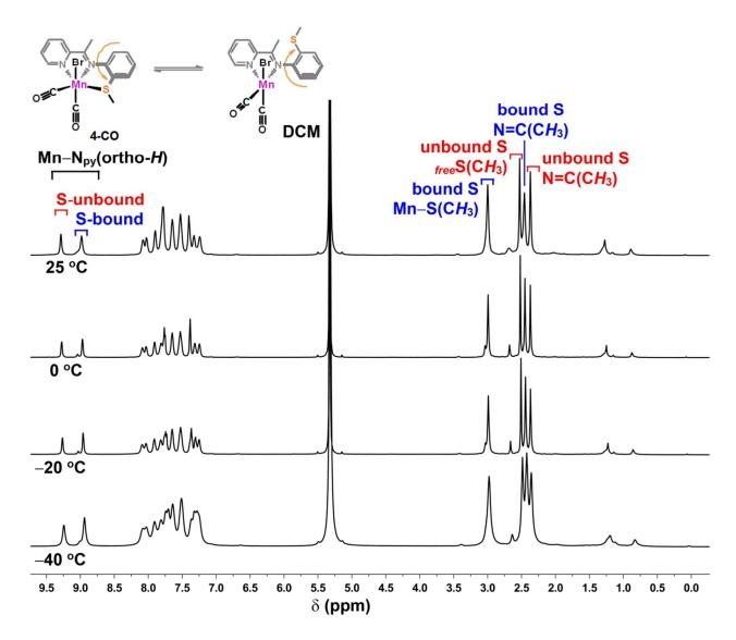
**Fig. 6.** Variable temperature  $^{1}$ H NMR spectra (500 MHz) of solution species derived from dissolving crystals of  $[(N_{Me}NS)Mn(CO)_{2}Br]$  ( $^{4}CO)$  in  $CD_{2}Cl_{2}$ .
