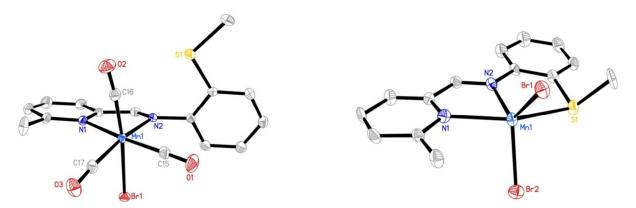
**Fig. 2.** ORTEP diagrams of the molecular structures of  $[(_{Me}NNS)Mn(CO)_3Br]$  ( $\mathbf{3}_{CO}$ , 50% ellipsoids) and  $[(_{Me}NNS)Mn(Br)_2]$  ( $\mathbf{3}_{Br}$ , 30% ellipsoids). H atoms are omitted for clarity.
