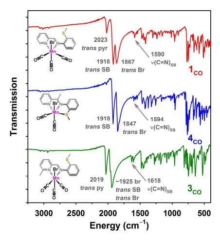
**Fig. 4.** Infrared spectra of  $[({}_{H}\underline{NN}S)Mn(CO)_{3}Br]$  ( $\mathbf{1}_{CO}$ , top red line),  $[(\underline{N}_{Me}\underline{NS})Mn(CO)_{2}Br]$  ( $\mathbf{4}_{CO}$ , middle blue line) and  $[({}_{Me}\underline{NN}S)Mn(CO)_{3}Br]$  ( $\mathbf{3}_{CO}$ , bottom green line) at 298 K in the solid state.
