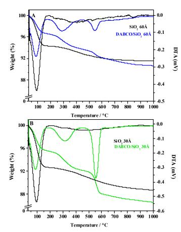
anchored DABCO/mesoporous SiO2 at 250-350°C and 540-580°C
