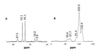
**Figure 3:** <sup>13</sup>C CP/MAS NMR (A) of the DABCO tether and the corresponding <sup>29</sup>Si CP/MAS NMR (B) spectra confirming the covalent link between the tether and the mesoporous silica support
