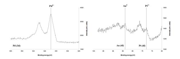
Figure 8 Pd (3d) XPS spectrum (*left*), and Au (4f) and Pt (4f) XPS spectra (*right*)obtained fromthe 2.28 wt% Au-2.28 wt% Pd-0.45 wt% Pt/TiO2 trimetalliccatalyst.
