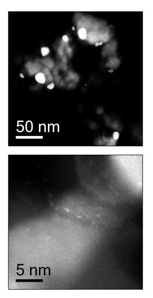
Figure 1 Representative STEM-HAADF images of the 2.50 wt% Au-2.50 wt% Pt/TiO<sub>2</sub> bimetallic catalyst. The low magnification micrograph (*left*) shows the presence of large nanoparticles ca 20 nm in diameter, whereas the higher magnification micrograph (*right*) shows that sub-nm clusters are also present.
