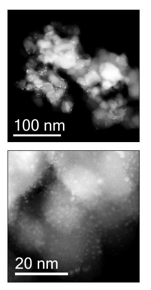
**Figure 5** Representative low (*left*) and high (*right*) magnification STEM-HAADF images of the 2.40 wt% Au-2.40 wt% Pd-0.20 wt% Pt/TiO<sub>2</sub> trimetallic catalyst.
