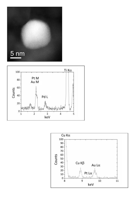
**Figure 6** STEM-XEDS analyses of the 2.40 wt% Au-2.40 wt% Pd-0.20 wt% Pt/TiO<sub>2</sub> trimetallic catalyst showing the typical compositions of smaller (*top*) and larger
