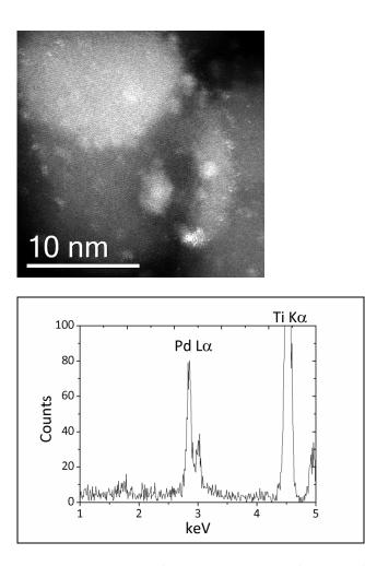
**Figure 7** Representative STEM-HAADF images of 0.20 wt% Au-4.60 wt% Pd-0.20 wt% Pt/TiO<sub>2</sub> trimetallic catalyst and the corresponding XEDS spectra obtained from these regions.
