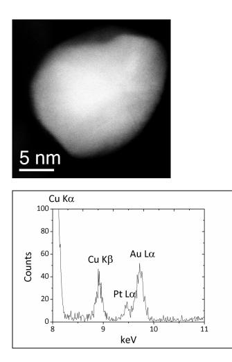
**Figure 2** STEM-XEDS analyses of the 2.50 wt% Au-2.50 wt% Pt/TiO<sub>2</sub> bimetallic catalyst, showing the typical composition of small (*top*), intermediate (*middle*) and large (*bottom*) size Au-Pt particles. A systematic composition /size variation was noted with the larger particles being Au-rich and the smaller ones being Pt-rich. Note the presence of Cu signal(s) in the XEDS spectra which represent an artefact from the support grid and are not characteristic of the catalyst samples.
