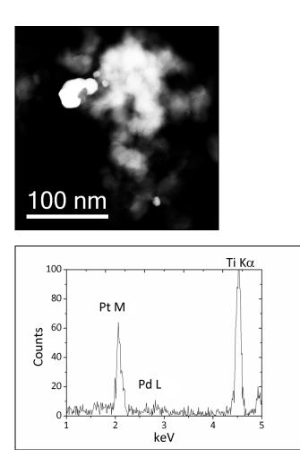
**Figure 4** STEM-XEDS analyses of the 2.50 wt% Pd-2.50 wt% Pt/TiO<sub>2</sub> bimetallic catalyst, showing the typical compositions of small (*top*), intermediate (*middle*) and large (*bottom*) size Pd-Pt particles. A systematic composition /size variation was noted with the larger particles being Pt-rich and the smaller ones being Pd-rich.
