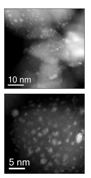
**Figure 3** Representative low (*left*) and high (*right*) magnification STEM-HAADF images of the 2.50 wt% Pd-2.50 wt% Pt/TiO<sub>2</sub> bimetallic catalyst.
