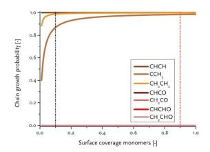
Fig 10 Computed chain-growth probability ( $\alpha$ ) as a function of the surface coverage of the chain propagating surface intermediate (CH in the carbide mechanism and CO in the CO insertion mechanism). The black and red dotted lines indicate typical respective C1 and CO coverage encountered under typical FT reaction conditions.
