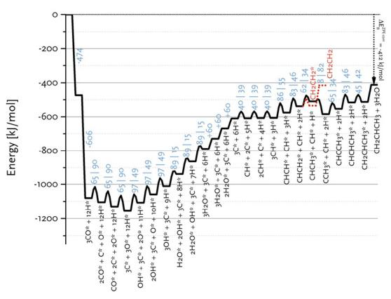
Fig 9 Reaction energy diagram for propylene from carbon monoxide and hydrogen. All data are for the  $Ru(11\overline{2}1)$  surface.
