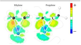
**Fig. 5** Electron density difference plots of the adsorbed states of ethylene (left) and propylene (right) on the Ru( $11\overline{2}1$ ) surface. These plots were generated by subtracting the electron density of the individual complexes in vacuum and empty surface from the electron density of the complex. Note that the electron density difference for ethylene is larger than for propylene.
