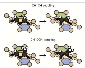
Fig 4b Schematic representation of CH-CH and CH-CCH $_3$  coupling on a step-edge site of the Ru(11 $\overline{2}$ 1) surface. The initial and final state of reaction are displayed.
