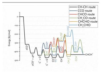
Fig. 8 Reaction energy diagram for CHCH\* formation from CO and  $H_2$ . The various routes in the CO insertion mechanism are compared to the CH-CH route in the carbide mechanism.
