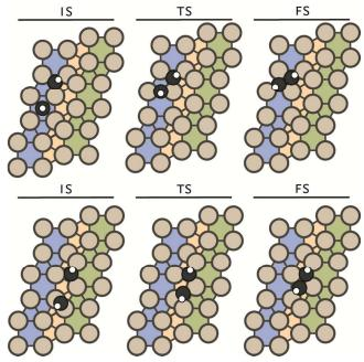
Fig. 2 Schematic representation of the two CH+CH coupling pathways on the  ${\rm Ru}(11\overline{2}1)$  surface. The coupling of two CH moieties on (top) a terrace site and (bottom) a step-edge site. The black and white spheres represent carbon and hydrogen atoms, respectively.
