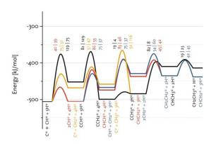
Fig. 7 Enlarged part of the reaction energy diagram showing various routes to ethane and ethylene formation. All data refer to the  $Ru(11\overline{2}1)$  surface.
