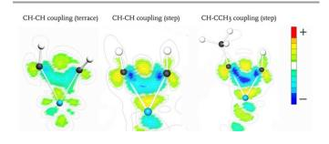
Fig 4a Electron density difference plots of the transition state for CH+CH coupling on the terrace (left), step-edge (middle) and of CH+CCH $_3$  coupling on the step-edge (right) of the Ru(11 $\overline{2}$ 1) surface. These plots were generated by subtracting the electron density of the individual CH moieties on the surface from the electron density of the complex. Note that the electron density difference for the step-edge site is larger than for the terrace site.
