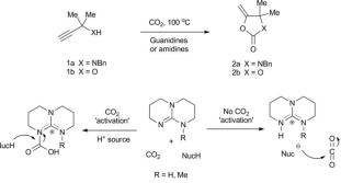
Scheme 2 Reaction between CO<sub>2</sub> and propargylamines and possible mechanisms with/without CO2 'activation'
