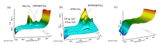
Fig. 1 Time evolution of ATR-FTIR spectra of reaction between CO<sub>2</sub> and THF solution of (a) TBD (7 mM); (b) MTBD (21 mM), followed by addition of water (2 x 6.6 eq.) and (c) TMG (8 mM), TEA (7 mM) or DABCO (9 mM). Data was collected every 30 seconds, at 8 cm<sup>-1</sup> resolution.
