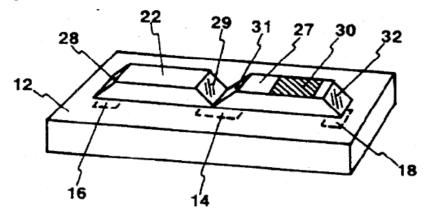
**Figure 27**. A smart waveguide sensor element for referenced indicator-based chemical sensing. Reprinted from ref.<sup>577</sup> Light from an LED (14) is directed by reflective end faces 29 and 31 into the two arms (22, 27; one acting as the sensor arm, the other as a reference) and then is reflected again (28, 32) to hit the detector (18) and reference detector (16), respectively. The sensing arm also contains a sensor layer (30) that affects the intensity of light passing it (27).
