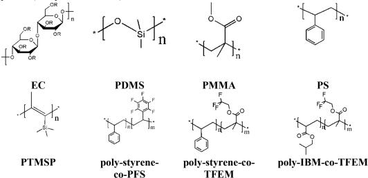
a) EC: ethyl cellulose; PDMS: poly(dimethylsiloxane); PMMA: poly(methyl methacrylate); PS: polystyrene; PTMSP: poly(1-trimethylsilyl-1-propyne); poly-styrene-co-PFS: poly(styrene)-co-(pentafluorostyrene); polystyrene-co-TFEM: poly (styrene)-co-(trifluoroethyl methacrylate); poly-IBM-co-TFEM: poly(isobutyl methacrylate)-co-(trifluoroethyl methacrylate); FIB: poly(hexafluoroisopropyl methacrylate)-co-(heptafluoro-n-butyl methacrylate); PSAN: poly(styrene-co-acrylonitrile).
