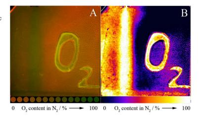
A similar approach has been reported by Park et al. In the first,<sup>585</sup> a light panel screen with light-emitting diode backlight was used as a light source to excite a sensor film containing PtOEP as the OSP in an ethyl cellulose host polymer. A green LED light uniformly displayed from the light panel
