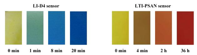
**Figure 5**. *Left*: Real color images of an irreversibly responding test stripe (consisting of a solution of leuco indigo in a polyurethane hydrogel; LI-D4) for oxygen over a time interval of 20 min. *Right*: Real color images of an irreversibly responding test stripe (consisting of a solution of leuco thioindigo in poly(styrene-co-acrylonitrile; LTI-PSAN) for oxygen over a time interval of 36 h. (Reprinted from ref. with permession from Elsevier)
