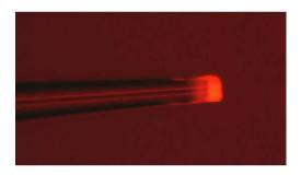
A configuration with crossed optical fibers was reported<sup>623</sup> that comprises silver nanoparticles covalently attached to the core of a fiber and labeled with luminescent ruthenium molecules. A second optical fiber (containing the ruthenium probe incorporated into nanoparticle) was placed at right angle of the first fiber to form a fiber-fiber junction. The system was used to detect the
