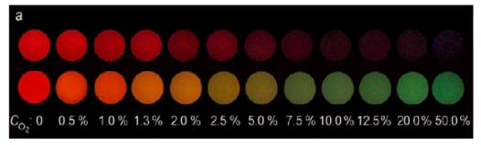
**Figure 15**. The apparent colors of luminescence colorimetric oxygen sensor without (upper) and with (lower) green-color background at different oxygen concentrations. (Reprinted from ref. 312 with permission from Wiley-VCH)
