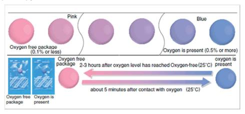
Figure 3. The color of Ageless Eye oxygen indicator changes from pink to blue in the presence of oxygen.
