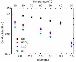
Figure 2: In-plane conductivity of the ETFE-g-PVBTMA AEM in HCO<sub>3</sub>-, CO<sub>3</sub><sup>2</sup>-, Cl<sup>-</sup> and OH<sup>-</sup> forms as a function of temperature at constant relative humidities; a) 95%RH and b) 80%RH
