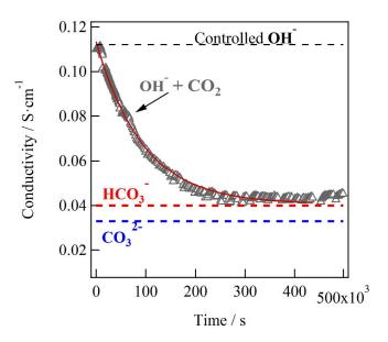
Figure 13: In-plane conductivity versus time of an ETFE-g-PVBTMA AEM initially in the OH form when exposed to compressed air in a RH and temperature controlled environment. Dotted lines represent the ionic conductivity of the AEM in pure anion forms. All measurements performed at 60°C and 95%RH. Solid red line corresponds to the fit of data with eqn. 15.
