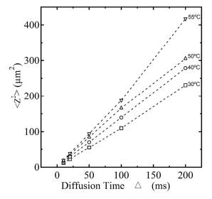
Figure 5: Mean squared displacements for fluoride ions as a function of diffusion time
