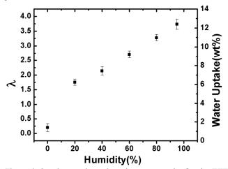
Figure 3:  $\lambda$  values and gravimetric water uptake for the ETFEg-PVBTMA AEM in the Cl form as a function of %RH at  $30^{\circ}$ C.
