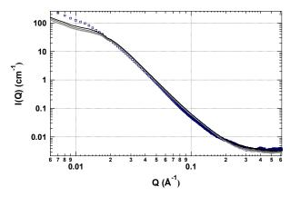
Figure 10: SAXS of the AEM with Cl<sup>-</sup> as the counter ion, at 60 °C, 25% RH, 50% RH, 75% RH and 95% RH light to dark, and boiled in 1 M KOH, at 60 °C, 95% RH, blue squares.
