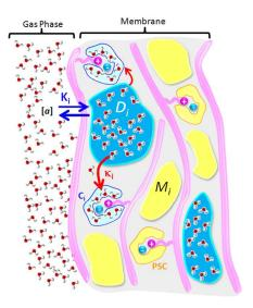
Figure 12: Schematic illustration of water interactions with various domains in the AEM.
