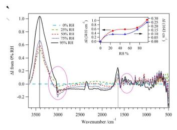
Figure 8: Difference FT-IR ATR spectra of the ETFE-g-PVBTMA AEM at various RH. The inset shows the dependence on water activity of the maximum intensity of both the 3110 cm<sup>-1</sup> (red circles) and 1643 cm<sup>-1</sup> (blue triangles) bands.
