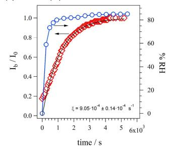
Figure 11: Dependence with time of the  $I_b/I_0$  intensity ratios (the intensity of the band at 3405 cm<sup>-1</sup>, v(OH) vibrational mode, respectively for the sample at t and at  $t = \infty$  s) and of the percent relative humidity (blue circles).  $I_b$  and  $I_0$  are intensity values measured at t=0 and  $t=\infty$  s, where t=0 s is time of gas flow change from dry to saturated  $N_2$ . Fit line corresponds to eqn. 10 that is derived in the main text below.
