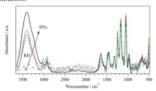
Figure 6: FT-IR ATR spectra of ETFE-g-PVBTMA AEMs at selected RHs between 0% - 95%. The spectra are normalized to the polymer backbone  $\delta(CH)$  peak at 1323 cm $^{-1}$  for presentation and analysis purposes.
