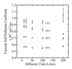
Figure 4: Self Diffusion Coefficient of  $F^-$  ions transport through the AEM at 100% RH as a function of diffusion time ( $\Delta$ )
