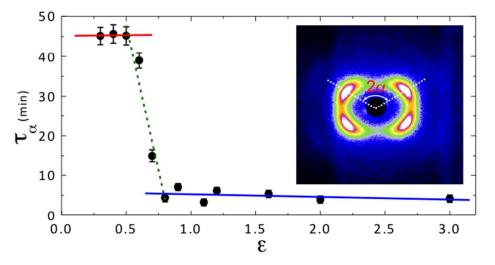
Relaxation rate of the chevron angle,  $\alpha$  becomes about ten times faster at higher strains exceeding 0.7 than at low strains.
