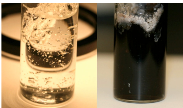
Figure 3. The initially colorless and optically transparent EDOT gels (left) change to a deep, dark bluish black (right, PEDOT gel) after the UV-initiated polymerization.
