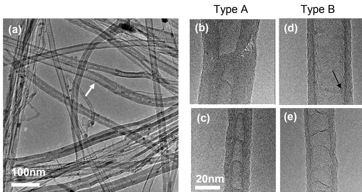
**Figure 1:** (a) An overview of the P,N-MWCNT sample showing the variation in nanotube structures. (b and c) Examples of nanotubes with a Type A morphology. (d and e) Examples of nanotubes with a Type B morphology. An example of amorphous material on the inner-wall of the nanotube is marked by an arrow in (d) (a larger version of the same nanotube is shown in the Supplementary Information, Figure S1).
