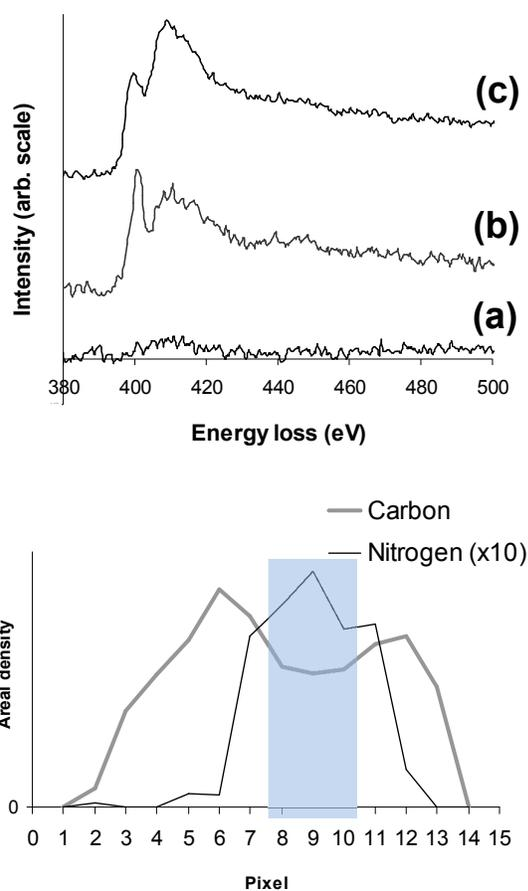
**Figure 3:** Nitrogen K-edge from (a) a Type A nanotube, (b) a Type B nanotube and (c) an irradiated Type B nanotube. (d) The variation
