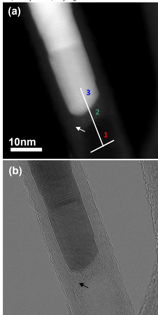
**Figure 4:** (a) HAADF and (b) bright field images of a Type B P,N-MWCNT containing a catalyst particle. The amorphous layer on the inside of the nanotube is indicated with an arrow in both images. The numbers 1, 2 and 3 in (a) indicate different regions of the line-scan.
