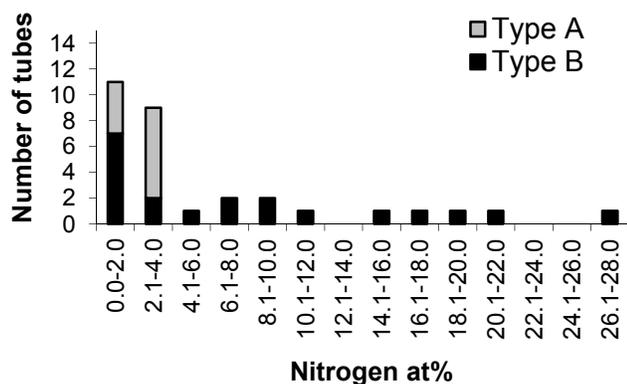
**Figure 2:** Nitrogen content of individual P,N-MWCNTs classified according to morphology.
