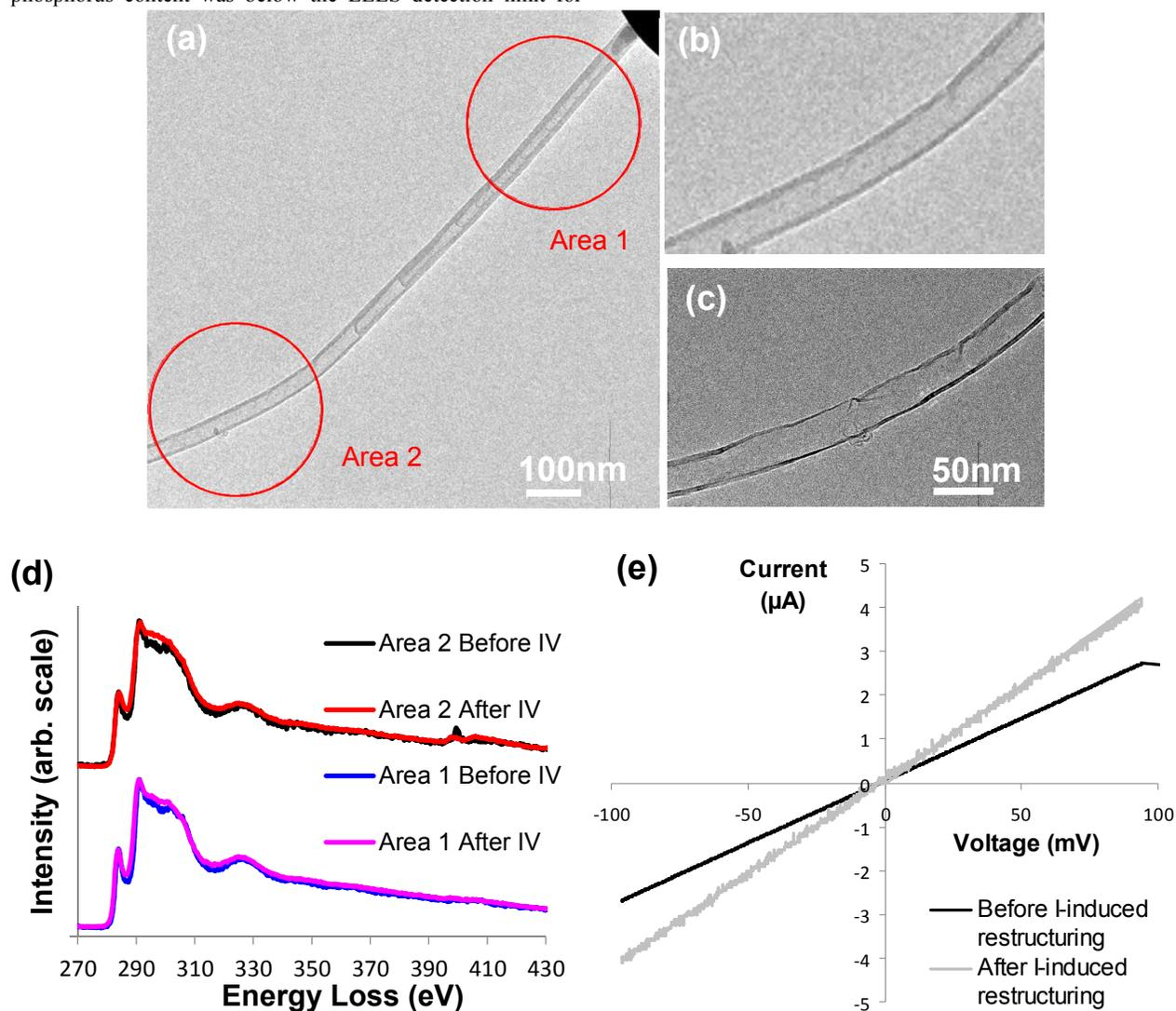
**Figure 5:** (a) P,N-MWCNT with a Type A (Area 1) and a Type B (Area 2) section. (b) Type B section before current flow. (c) Type B section after current flow. (d) EELS spectra of areas 1 and 2 before and after the initial  $IV$  spectra were taken. (e)  $IV$  curves before and after the current-induced restructuring of the nanotube.
