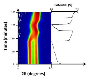
**Figure 8.** Selected 2 $\theta$  region of *in situ* synchrotron XRD data highlighting the evolution of the 200 reflections of the two FeCo(CN)<sub>6</sub> phases by a colour scale and the potential profile.
