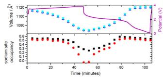
**Figure 6.** The evolution of the sodium site occupancy for the vacancy-free (black) and vacancy-containing models (red), and unit cell volume (blue and cyan for the vacancy-free and vacancy-containing models respectively) of the major  $\sim$ Na<sub>0.5</sub>FeFe(CN)<sub>6</sub> phase as a function of time, with the potential profile included.
