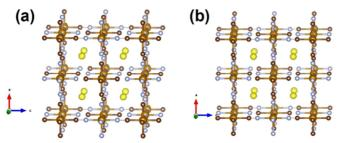
**Figure 5.** The crystal structure and remaining Fourier electron density (yellow) of the major  $\text{FeFe}(\text{CN})_6$  phase in the 2<sup>nd</sup> battery, with iron in light brown, carbon in dark brown and nitrogen in blue. (a) and (b) show the vacancy-free and vacancy-containing models respectively.
