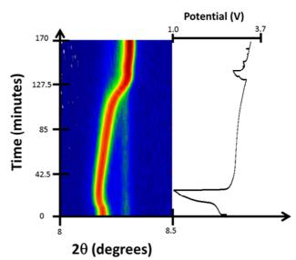
**Figure 3.** Selected  $2\theta$  region of *in situ* synchrotron XRD data highlighting the evolution of the 200 reflections of the two FeFe(CN)<sub>6</sub> phases by a colour scale and the potential profile.
