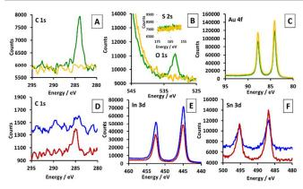
Figure 5. X-ray photoelectron spectra (XPS) of solution processed Au cathodes detecting the surface (green) and sub-surface (yellow) presence of carbon [A], oxygen [B], sulphur [B inset] and gold (0) [C] and the content of carbon [D], indium (III) [E] and tin (IV) [F] of sub-surface commercial ITO (blue) and solution processed ITO (red).
