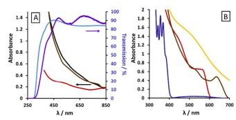
Figure 3. UV-Vis transmission of commercial ITO (light blue) and ITO-sol (purple) on glass and absorption of CdSe-sol (red), CdTe-sol (brown) and CdSe-sol/CdTe-sol films together (black) on commercial ITO glass substrates [A], and absorption of nanocrystal precursor solutions of CdSe (red), CdTe (brown), Au (gold), and ITO (purple) prior to annealing [B].
