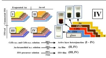
**Scheme 1.** Deposition scheme of four device architectures starting with solution processing of only the nanocrystal (n.c.) active layers with the typical pristine evaporated ITO and Au contacts [I], with Au-sol contact [II], with ITO-sol contact [III], and the all-solution device [IV] including photos of each precursor solution.
