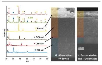
Figure 2. XRD patterns of each individual layer of ITO-sol [A], CdSe-sol [B], CdTesol [C], and Au-sol [D] and the completed cell (x2.0 intensity for clarity) containing each layer as ITO-sol/CdSe-sol/CdTe-sol/Au-sol [E] including a cell with evaporated contacts as ITO/CdSe-sol/CdTe-sol/Au [F] and cross-section SEM images of the all-solution device (Device IV) [G] and the device built with evaporated contacts (Device I) [H].
