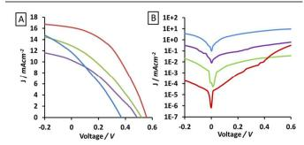
**Figure 4.** Measured light J-V curves for representative solar devices [I] (red), [II] (green), [III] (blue) and [IV] (purple) which are  $0.1 \text{ cm}^2$  masked device squares formed from the intersection of ITO and Au contacts and illuminated through the ITO-glass side under AM 1.5G filtered spectral illumination (100 mWcm<sup>-2</sup>) [A], and the dark JV curves for the same devices [B].
