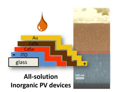
**TOC:** Robust all inorganic solar cells showing 1.7% efficiency were fabricated entirely from solution in air onto non-conductive glass using solution soluble nanocrystal inks.
