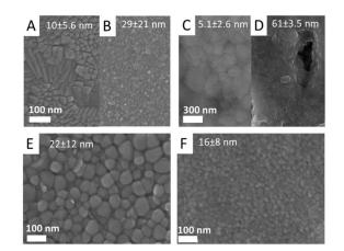
**Figure 1.** SEM images with RMS roughness values (nm) of commercial ITO [A] and ITO-sol [B] bottom electrode films on glass, evaporated gold [C] and Au-sol [D] top contacts, with CdTe-sol [E] and CdSe-sol [F] active layer films.
