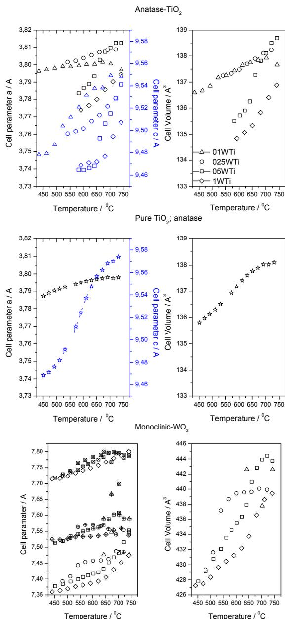
Fig. 7. Cell parameters and volume for the anatase-TiO<sub>2</sub> (a,c) and monoclinic-WO<sub>3</sub> (a<b<c) phase as obtained from Rietveld analysis of XRD data taken during an O<sub>2</sub>/He temperature ramp. The Ti reference system is presented in separated plots.
