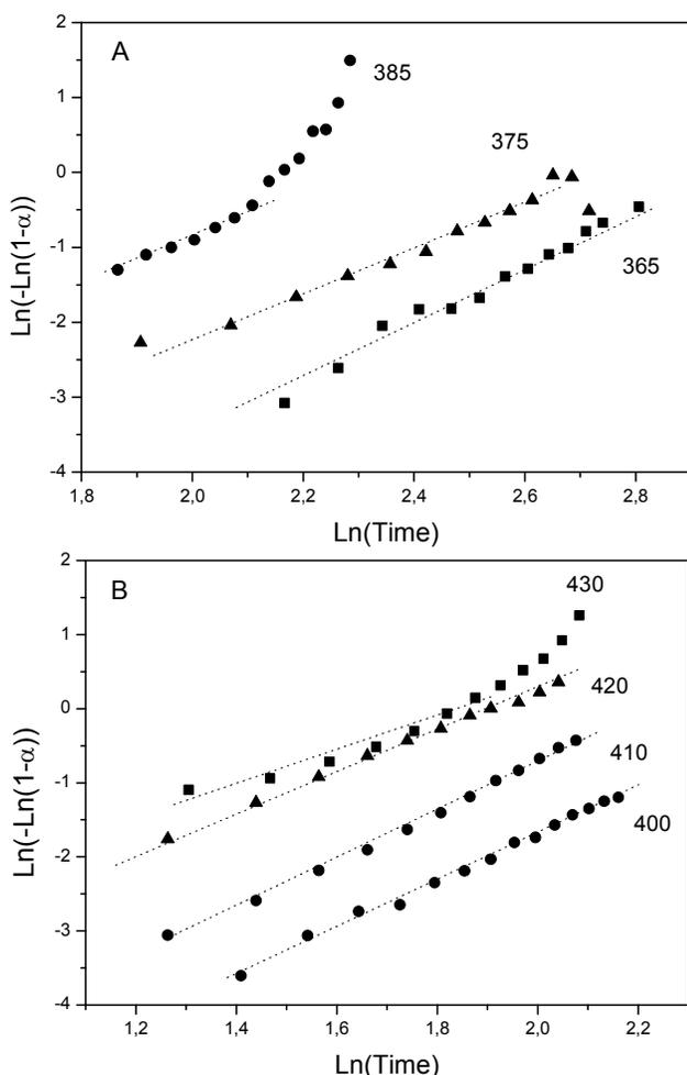
Fig. 4. Sharp- Hancock plots (equation 1) for the T (A) and 025WTi (B) samples. Numbers indicates the temperature ( $^{\circ}\text{C}$ ) of the isothermal treatment. Linear fittings are presented as dotted lines.
