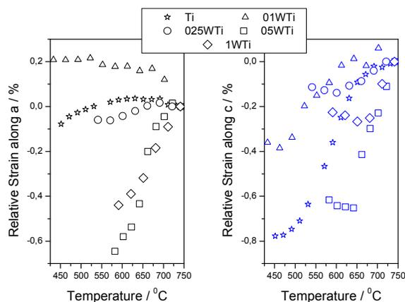
Fig. 8. Evaluation of the strain present in the anatase unit cell during a O<sub>2</sub>/He temperature ramp. Thermal effects eliminated as described in the text. Strain is defined as  $(p_i - p_{\text{final}}) / p_{\text{final}} \times 100$ , where *p* is the corresponding anatase cell parameter.
