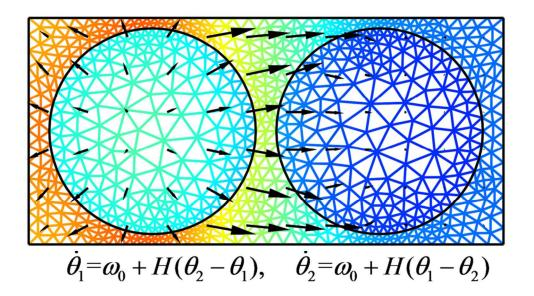
Further explanation of excitatory and inhibitory coupling between Belousov-Zhabotinsky droplets with three levels of modeling (point, finite element and phase). 40x25mm (600 x 600 DPI)
