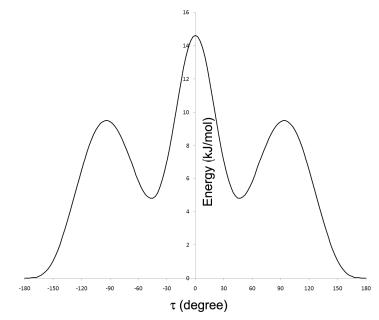
**Figure 5**. Energy of 3-CINA single molecule as a function of torsion angle  $\tau$  in relative to the lowest-energy conformer.
