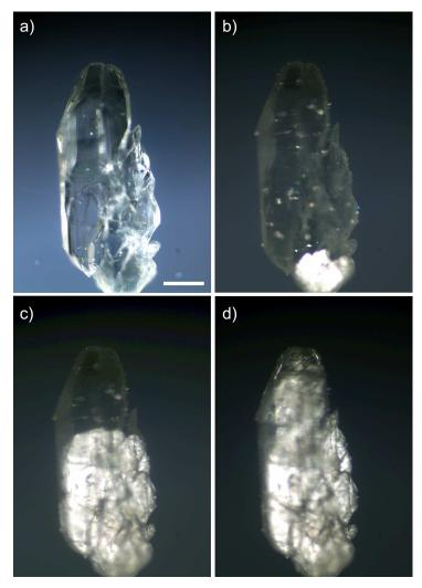
**Figure 7**. Solid-to-solid phase transition of form II to form I observed by hot-stage microscopy during heating: 91.2 (a), 133.0 (b), 134.4 (c), and 135.7 °C (d). Scale bar: 0.2 mm.
