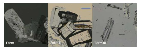
**Figure 2**. Crystals of the three polymorphs (I, II and III) of 3-CINA. Scale bar: 0.3 mm.
