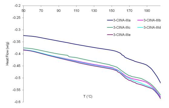
Figure 10. DSC thermograms of form III (five repeats).
