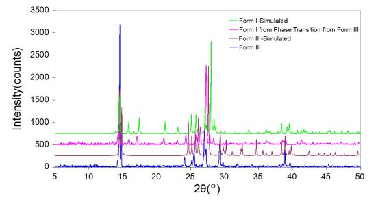
Figure 9. PXRD of form III before and after the solid-to-solid phase transition.
