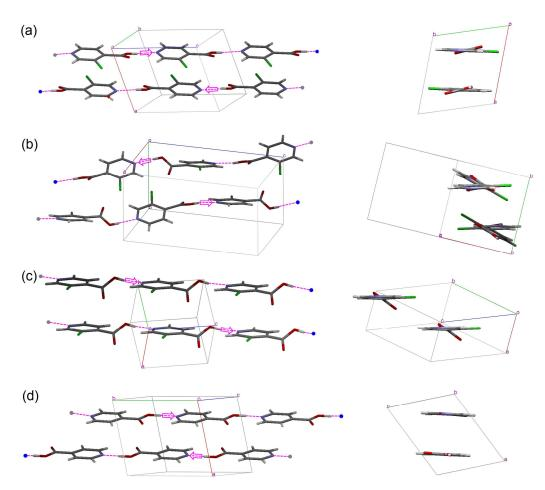
**Figure 4**. Different views for crystal packing of forms I (a), II (b), III (c) of 3-CINA, and isonicotinic acid (d). Hydrogen bonds are highlighted with dash lines, and the arrows indicate the hydrogen-bonding directions (from donor to acceptor).
