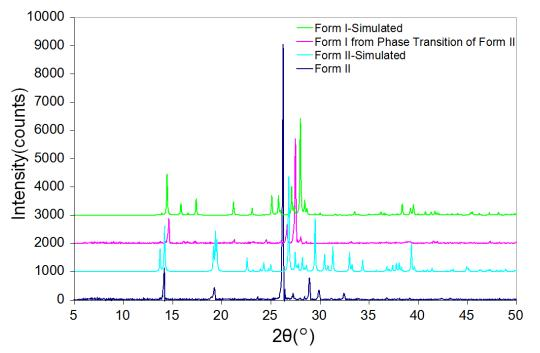
Figure 8. PXRD of form II before and after the solid-to-solid phase transition.
