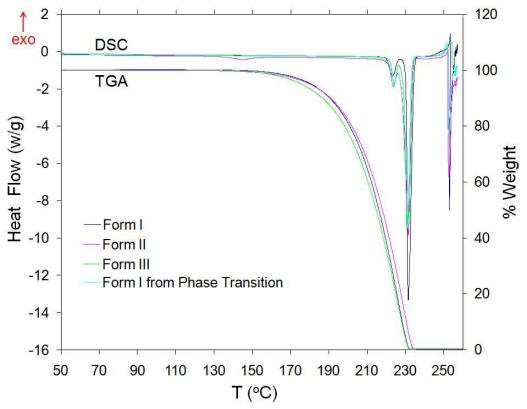
**Figure 6**. DSC and TGA thermograms of the three polymorphs. TGA were run in open DSC pans. Form I converted from form II is also shown in DSC.
