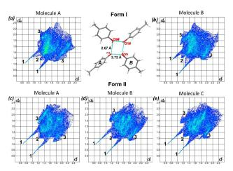
Fig. 5 2D fingerprint plots of (a) form I – molecule A, (b) form I -<sup>55</sup> molecule B, (c) form II - molecule A, (d) form II - molecule B and (e) form II - molecule C. The close contacts are labelled 1-3 where 1 is H•••O, 2 is H•••H and 3 is C•••H.
