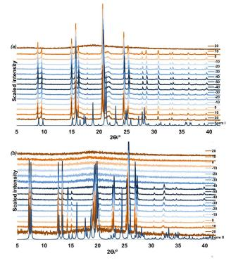
Fig. 4 VTPXRD study for *in situ* crystallisation of (a) from top: form I recorded at 10°C intervals, ten minute equilibration was allowed after
