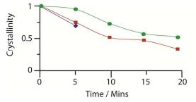
Figure 4: Evolution of the crystallinity of rho-ZMOF after milling for increasing amounts of time. Blue- evacuated, red - ethanol containing, green - butanol containing
