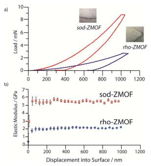
**Figure 2**: Representative (a) load vs displacement curves and (b) elastic moduli values as a function of depth for **1** and **2**. Error bars are taken from the standard deviation of more than 15 indents.
