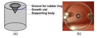
**Fig. 2** (a) A Schematic diagram of the growth cell; (b) The mounting plate with an inserted growth cell.
