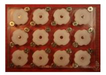
**Fig. 4** A plate of  $4 \times 3$  cells for ceiling crystallisation.
