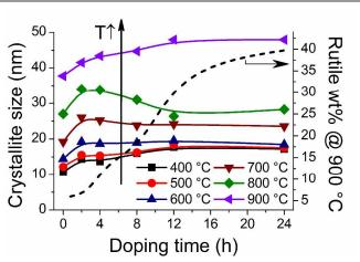
Figure 4. Variation of the anatase crystallite size with nitrogen doping under different calcination conditions (left axis), and the rutile weight fraction in the sample calcined at  $900^{\circ}C$  (right axis). Lines are guides for the eye.
