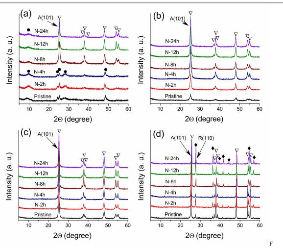
Figure 3. Variation of the XRD pattern of TiONTs before heat treatment (a) and calcined at 400 °C (b), 600 °C (c) and 900 °C (d). Reflections assigned to trititanate nanotubes " $\bullet$ ", anatase " $\nabla$ " and rutile " $\bullet$ " are indicated in each panel.
