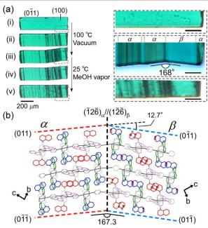
**Fig. 3** (a) Bending and straightening process of **1** observed under a polarized microscope. The right figures are enlarged images of the marked portions of the left images of i, iii, and v (scale bars in enlarged figure are 30  $\mu$ m). (b) Connection of packing structures of  $\alpha$  and  $\beta$  phases on the interface.
