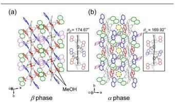
**Fig. 2** Packing structures of (a)  $\beta$  phase (**1**•MeOH) and (b)  $\alpha$  phase (**1**) viewed along each *c* axis. Inset figures represent the bending angle of zigzag 1D chains.
