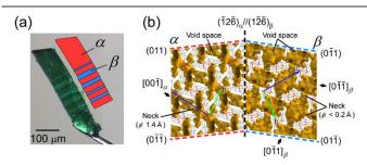
**Fig. 4** (a) Single crystal of **1** under  $\alpha$ - $\beta$  coexisting state used for crystal face indexing. (b) Connections of pore structures on the interface. (Yellow regions are void spaces.) The necked channels in the center of the  $\alpha$  phase are blocked by the two neighboring  $\beta$  phases on each interface whereas the channels near the edge of the  $\alpha$  phase reach the crystal surface of (011) $_{\alpha}$  or (0-1-1) $_{\alpha}$ .
