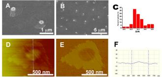
Fig. 2 Changing the morphology of bi-compartmental particles by deposition from acetone: A, B) SEM images showing the bright spots to be off-center compared to the dark parts; C) analysis of the deviation of centers of the bright parts (R is the radius of the whole particle while D is the distance between the centers of the bright and dark parts); D, E) AFM height and phase images of a particle; F) AFM height profile of the line scan shown in D.
