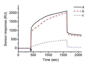
Figure 1. SPR sensorgrams of CB[7] SAM treated with a) FA-TBA, b) FA-SDNA and c) TBA (The arrow indicates injection of samples)
