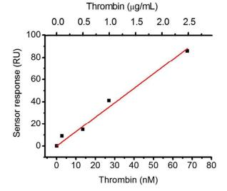
Figure 2. Sensor responses as a function of thrombin concentration on CB[7] SAM SPR sensor chip (15 min. 5 μL/min)
