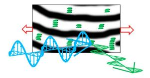
Composite materials obtained by doping a SBS thermoplastic elastomer matrix with CdSe nanoplatelets show reversible platelets alignment upon stretching.
