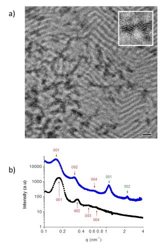
*Figure 2.* Structure of the hybrid material. a) TEM image of the composite film. Scale bar is 50 nm. Inset is a  $3 \times$  magnification on NPLs. b) SAXS diagram of a pure SBS film ( $\blacksquare$ ) and of the composite film ( $\blacktriangle$ ). The reflections arising from the lamellar microstructure of the SBS template are indicated in red whereas the reflections due to the NPL stacking are indicated in green.
