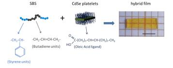
*Figure 1.* Components of the hybrid film. Left: schematic representation of a SBS copolymer chain. Center: schematic representation of a CdSe nanoplatelet covered with ligands. Right: photography of the hybrid film (Scale bar is 2 mm).
