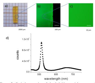
*Figure 3.* Optical properties of the hybrid material at rest. a) Photograph of the composite film and b) and c) optical fluorescence microscopy images of the same film with FITC filter, at different magnifications. d) Fluorescence spectrum of the same film with excitation at 400 nm.
