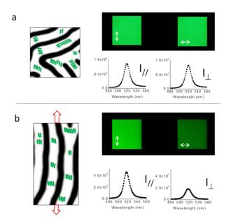
*Figure 5.* Effect of stretching on the fluorescence properties of the hybrid material: schematic representation of a composite film, optical microscopy and emission spectra of, a) film at rest showing isotropic photoluminescence; b) stretched film (100% strain) showing anisotropic photoluminescence. The white arrows represent the direction of the analyzer.
