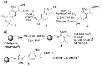
Scheme 1. (a) Synthesis of the photocleavable linker 3. (b) Immobilization of the photocleavable NPPOC derivative 3 onto PS solid support (NittoPhase®).
