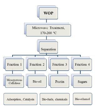
**Figure 4**. Scheme of microwave hydrothermal pyrolysis of waste orange peel. WOP stands for waste orange peel. [Adapted from Ref.14, with kind permission].
