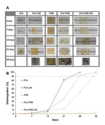
**Figure 7**. Appearance of film samples before and after different days of disintegration under composting conditions (A). Film samples with *d*-limonene (PLA–LIM and PLA–PHB–LIM, *bottom*) disintegrate much faster than their counterparts without *d*-limonene (PLA and PLA–PHB). [Image reproduced from Ref.45, with kind permission].
