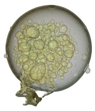
**Figure 9**. X-ray micro-tomography image of a *Ceramisphere* (a trademark of Ceramisphere Pty Lrd) containing encapsulated limonene. [Photo courtesy of Dr Sherry Mayo, ANSTO, reproduced with kind permission of Ceramisphere].
