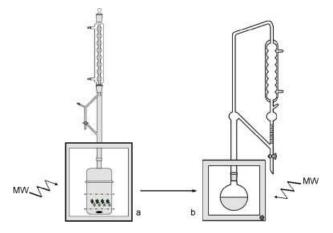
**Figure 6**. Proposed extraction procedure using limonene: microwave-integrated Soxhlet extraction (a) followed by microwave Clevenger distillation (b). [Image reproduced from Ref.27, with kind permission].
