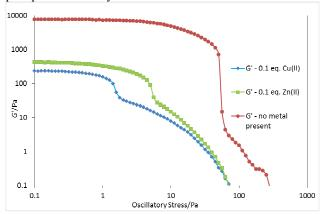
Figure 3. Stress sweep rheometry data for a 1 wt. % hydrogen of compound **1a** in the presence of Cu(NO<sub>3</sub>)<sub>2</sub> and ZnCl<sub>2</sub> compared to the pure compound.
