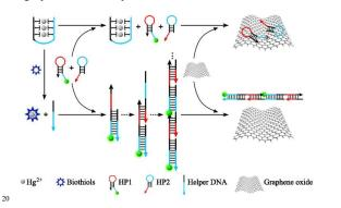
**Scheme. 1.** Illustration of GO based platform couple with hybridization chain reactions for biothiol analysis.
