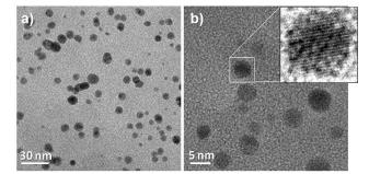
Fig. 3 TEM images of (a) PS<sub>191</sub>-P4VP<sub>280</sub>/AuNP after heating in 1,4-40 dioxane at 160°C (under pressure) for 20 h, (b) PS<sub>192</sub>-P4VP<sub>162</sub>/CuNP after heating in 1,4-dioxane at 105°C for 20 h.
