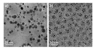
Fig. 5 TEM images of  $PS_{398}$ -P4VP<sub>166</sub>/CuNP after heating in 1,4-dioxane at 160°C for 20 h. Metal to VP ratio is (a) 1:1, (b) 10:1. Dashed circles in b highlight the boundaries of micelle cores (P4VP) with CuNP inside.
