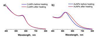
Fig. 2 Normalized UV-vis spectra of (a)  $PS_{192}$ -P4VP<sub>162</sub>/CuNP and (b)  $PS_{191}$ -P4VP<sub>280</sub>/AuNP before and after heating in 1,4-dioxane at 160°C for 15 20 hours.
