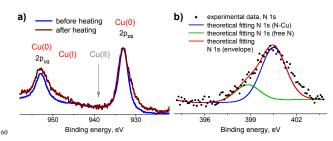
**Fig. 4** XPS of PS<sub>192</sub>-P4VP<sub>162</sub>/CuNP: (a) copper 2p XPS spectrum region before and after heating in 1,4-dioxane at 105°C for 20 h; (b) nitrogen 1s XPS spectrum region (before heating).
