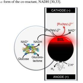
**Scheme 1** Illustration of enzyme-driven ECL observed on a bipolar swimmer. Glucose is oxidized by glucose dehydrogenase (GDH) with NAD<sup>+</sup> as a co-factor. The enzymatically-produced NADH behaves as an 70 *in situ* co-reactant for the ECL generation.
