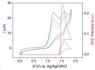
**Fig. 1** Cyclic voltammograms (blue lines) and ECL signals (red lines) of 1.5 mM Ru(bpy)<sup>3+</sup><sub>3</sub> in the presence of 10 U.mL<sup>-1</sup> GDH, 10 mM NAD<sup>+</sup> and various glucose concentrations (5 mM, dotted lines; 10 mM, dashed lines and 40 mM, solid lines) in 100 mM PBS solution (pH 7.4). A GC <sup>35</sup> electrode (same material as the swimmer) was used to record both CV and ECL. Scan rate 0.05 V.s<sup>-1</sup>.
