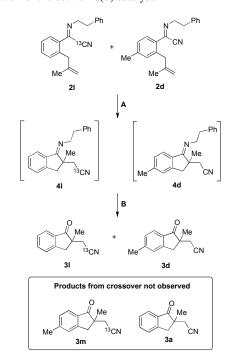
A: Pd(PPh<sub>3</sub>)<sub>4</sub> (15 mol %), ZnCl<sub>2</sub> (20 mol %), PhMe, 120 °C, 24 h B: AcOH, rt, 12 h Scheme 3: Crossover Experiment
