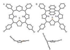
Figure 2. The X-ray molecular structures of *m*-Bpor (A) and Apor (B) (top: perspective view, bottom: side view with aryl groups omitted for clarity)
