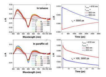
Figure 4. The TA spectra (left) and decay profiles of *p*-Bpor in toluene (top) and paraffin oil (bottom)
