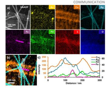
than the dry reference spectra. Only through the use of the elemental spectrum images is it possible to unambiguously interpret the HAADF image to distinguish the compositional distribution of the individual nanostructures present. From the XEDS data, it is clear that there are two ~40 nm diameter Au-NPs on either side of the image and that the Pd-CNT contains a distinct residual Fe catalyst core. The
