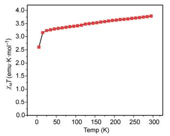
Fig. 3 Temperature dependence of  $\chi_M T$  for 1-FeCl<sub>2</sub>, obtained under a 1000 Oe measuring field. Line added only as a guide for the eye.
