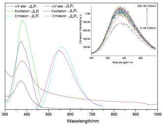
**Figure 2**. The UV absorption, excitation (JLP<sub>1</sub> - $\lambda_{em} = 545$  nm and  $\lambda_{em} = 560$  nm) and emission spectra ( $\lambda_{ex} = 405$  nm) of JLP<sub>1</sub> and JLP<sub>2</sub> in aqueous solution. Inset: The emission enhancement of JLP<sub>2</sub> upon the addition of the 200 nM EBNA1.
