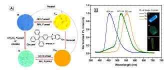
**Fig. 1** A) Molecular structure of TPENSOH and fluorescence images of the powders: (B<sub>1</sub>) as-prepared TPENSOH; (G<sub>1</sub>) ground sample; (Y<sub>fa1</sub>) B<sub>1</sub> in the vapor of HCl for 10 min; (O<sub>fa1</sub>) G<sub>1</sub> in the vapor of HCl for 10 min. (Excitation 70 wavelength: 365 nm). B) PL spectra of the three single crystals. The insets depict the fluorescence microscope images of the single crystals. (Excitation wavelength: 365 nm).
