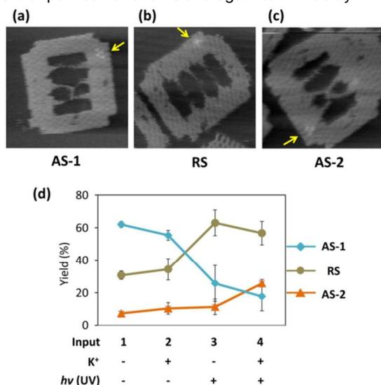
**Fig. 3** AFM images of three states and the yield of them under four independent inputs. **Input-1:** without any stimulation; **Input-2:** under buffer containing 50 mM  $K^+$ ; **Input-3:** UV irradiation for 10 min at 35 °C; **Input-4:** integrating 50 mM  $K^+$  with UV irradiation for 10 min at 35 °C. The hairpin marker was pointed out by yellow arrow. The experiments were all repeated three times, and the error bars represent S.D. Image size: 150 nm × 150 nm.
