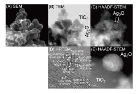
Fig. 2. SEM (A), TEM (B), HR-TEM (D), and HAADF-STEM images (C, E) observed for as-prepared Ag-TiO2 photocatalyst stored in ambient
